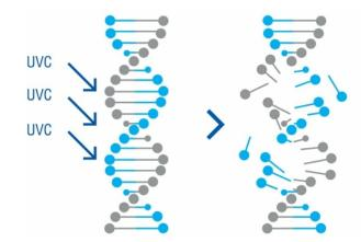
UV-C band ultraviolet energy, at the wavelength of 254nm, inactivates microorganisms at a molecular level by damaging their DNA structure.
